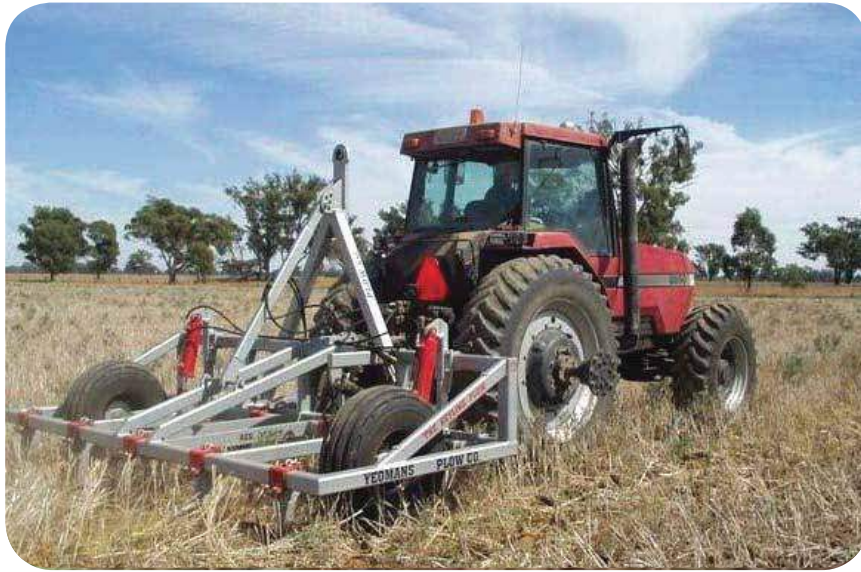
L65-11, Trailing Model / Linkage Plow fitted with 26" Shanks.
