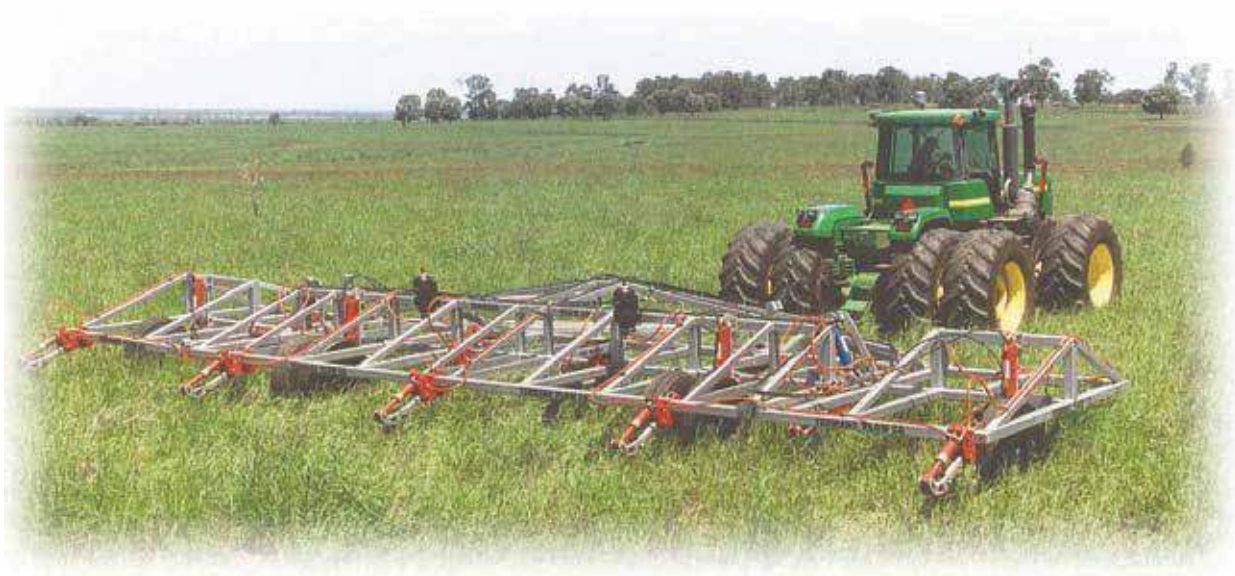
"40" foot (12.2m) Folding Wing Model set up with thirteen Stump Jump Shanks. West of Biloela in central Queensland".
