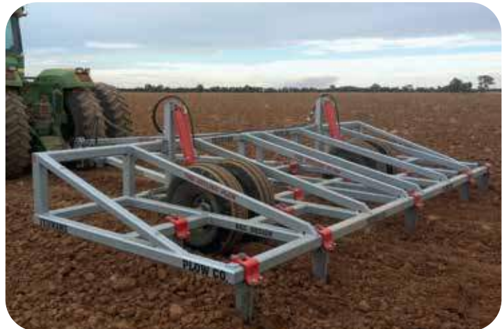
T92-21 with 26" shanks and dual 11.00x16 wheels.
