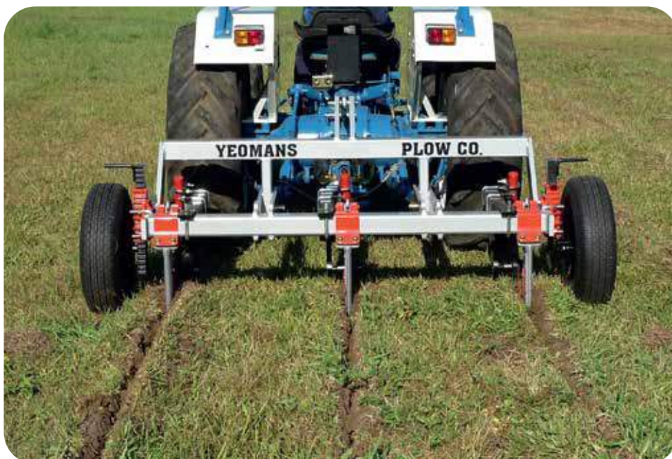
SB-6 pasture renovating with three 22" shanks; 16" pasture coulters and depth control wheels
