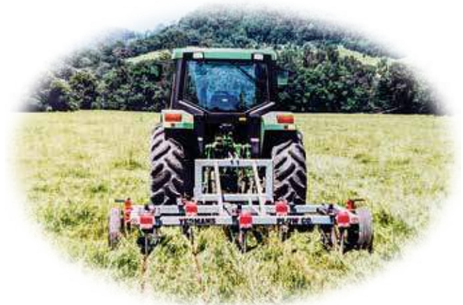
L43-10 with five 26" Shanks and 18" Coulters subsoiling to help improve this pasture.
