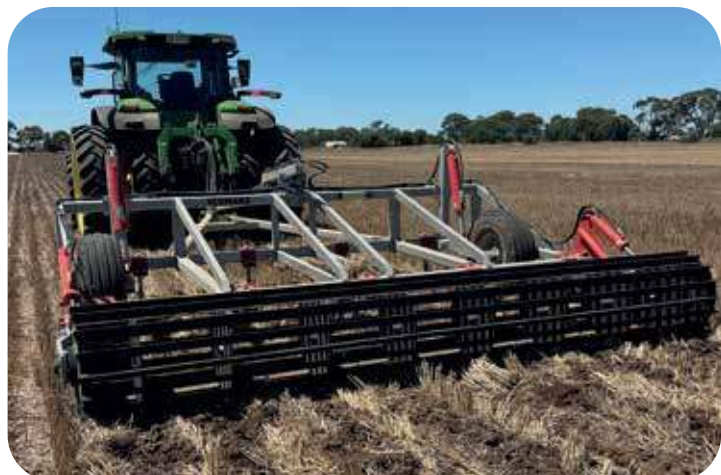
T74-14LD with 26" shanks single 11.00x16 wheels and Hydraulic height adjust Crumble Roller.
