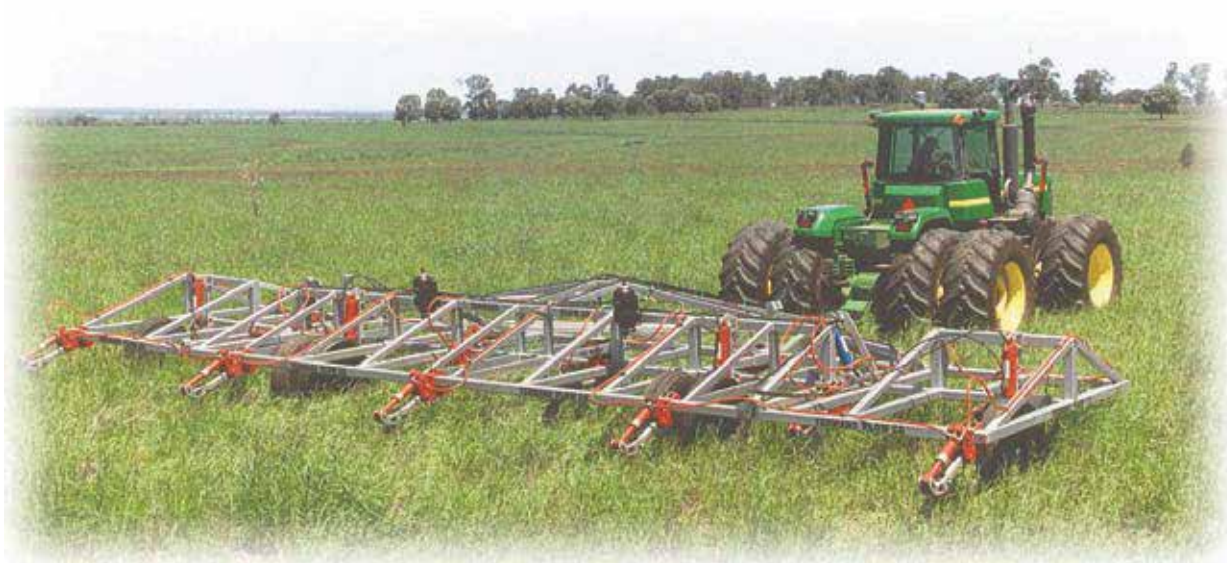
"40" foot (12.2m) Folding Wing Model set up with thirteen Stump Jump Shanks. West of Biloela in central Queensland".
