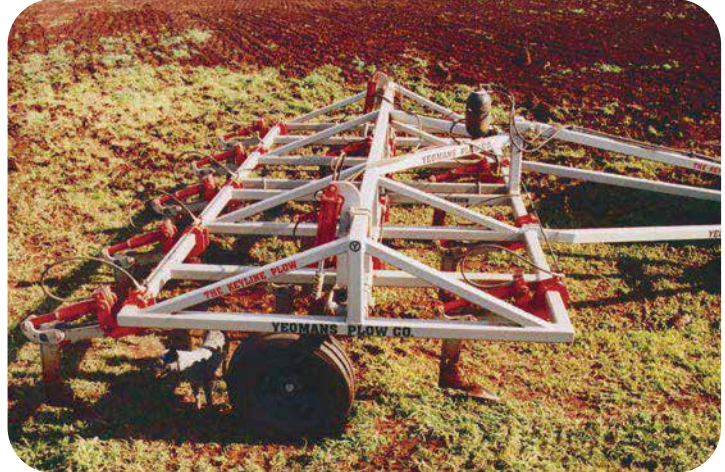
T123SJ-15 with thirteen Stump Jump Shanks at 13" spacing.
