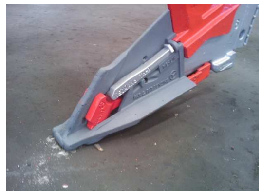
ML-1 [SJ] POINT WITH COLLOIDAL BORON CARBIDE HARDFACING FOR STUMP JUMP APPLICATIONS,
