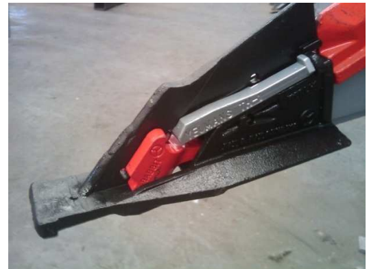
ML-1 [CBC] POINT WITH COLLOIDAL BORON CARBIDE HARDFACING FOR ROCKY CONDITIONS
